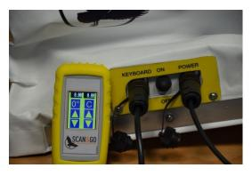
Pressing the button with the indication  $0^{\circ}$ , the system proceeds automatically reaching the horizontal plane on both axes.
